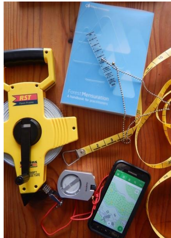
Basic tree survey tools: Map/GPS (in this case a mobile phone setup with Viewranger), Suunto clinometer, 25m tape measure, Cruiser's Crutch relascope, Forest Mensuration handbook, girth tape. You should also consider safety glasses if working in dense stands, and paint or timber chalk may be useful to mark trees already measured.
